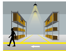
After hold time, lighting dims if no further movement is detected
