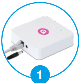
1 Connect Hub to Internet router and power
